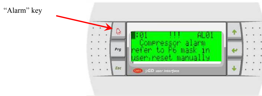
Fig.- 30 Screen status when alarm reported
